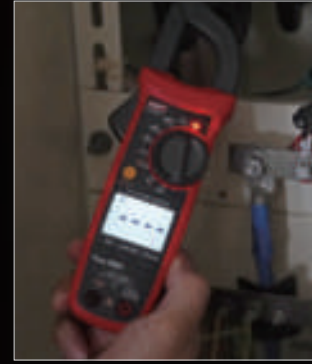
NCV multi-segment display and audio/visual alarm
